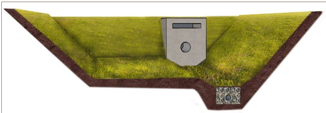
Exhibit 3. Alternative B: floodplain detention system concept for Arguello Park
