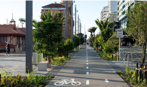
Figure 91 Quay Street in Auckland is an example of using street furnishing and landscape to delineate a sidewalk and Class I Bikeway.
