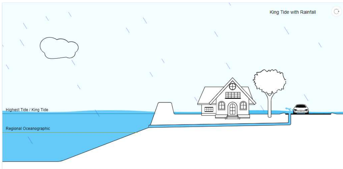
Exhibit 3. Tidal limitations on stormwater drainage and flooding. Graphic by (NOAA, 2024)
